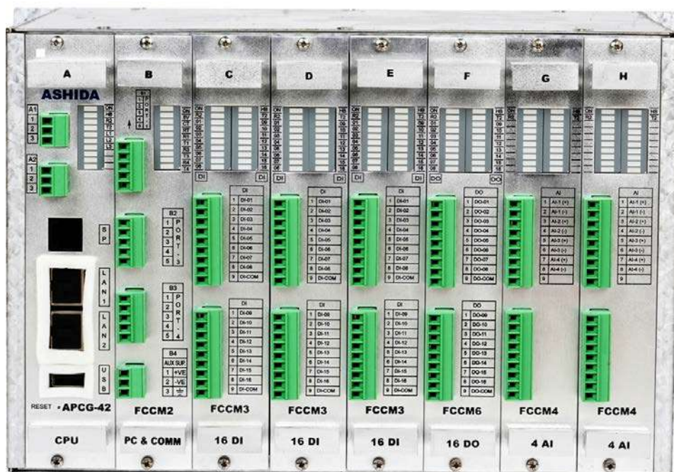
ASHIDA Feeder Remote Terminal Unit (APCG – 42)
