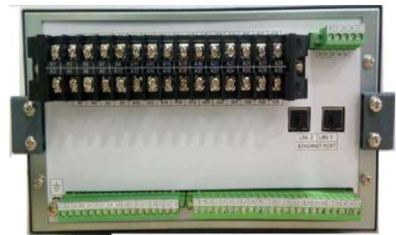
Back side terminal details: Plug-In
