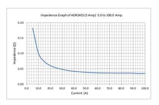
From impedance Graph, the maximum Voltage required across the relay terminal at fault current of 20 times of rated:
